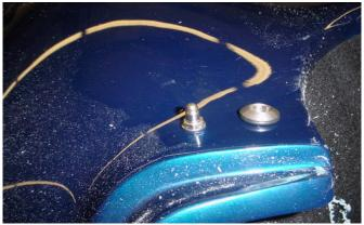
h. Measure 2.875" from inside lip of trunk towards the back of the cockpit, and the center of the trunk measured between the trunk hinges. Drill a 5/32 hole here and install the center rear lift the dot stud.
