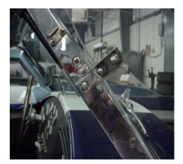
Step 5: Assemble Top Frame on Car
