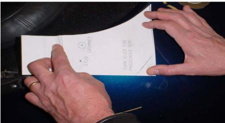
Locate the template on the driver's side and mark the 29/64" hole for the  $\frac{1}{2}$ -20 tap, and the 5/32 hole for the lift the dot stud. Turn the template over and repeat for the passenger side
