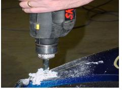
c. Drill the 5/32" hole for the lift the dot stud
